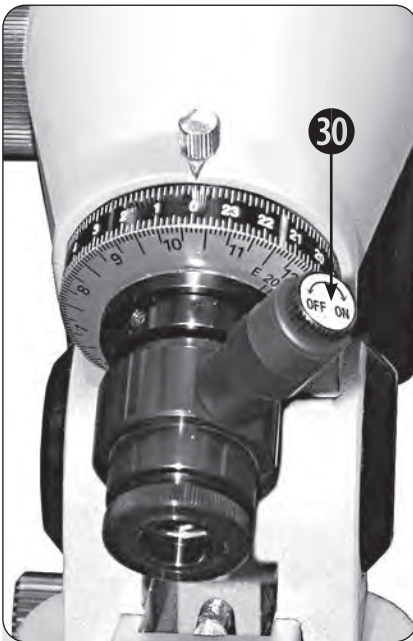
Fig. 37: Detailed view: polar finder with rotary knob (ON/OFF)
