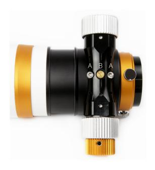
A: M4 screws for attaching the focuser retrofit. NOTE: DO NOT adjust it before asking W.O.
