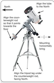
Fig. 3 The parallactic home position, side view
