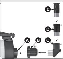
Fig. 1: Assembly sequence of optical accessories on the focusing unit (A) - here using the example of a Maksutov-Cassegrain telescope: Nut/retaining ring (B, optional), zenith prism (C), Barlow lens (D), eyepiece (E)
